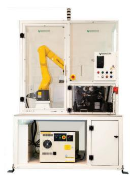
The RPA6000 ships as a complete system ready to be positioned against the conveyor system to begin applying labels with a minimum of effort.
